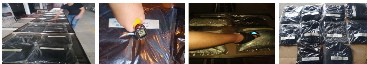
Figure 1 – Radiation treatment of samples at 400 kGy in an inert gas mixture (nitrogen and carbon dioxide in a ratio of 1/1)
